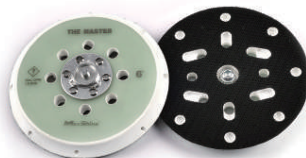
3011150P 6" (150mm) Max OPM: 12000 Thread: 5/16"-24 Hole: 8
